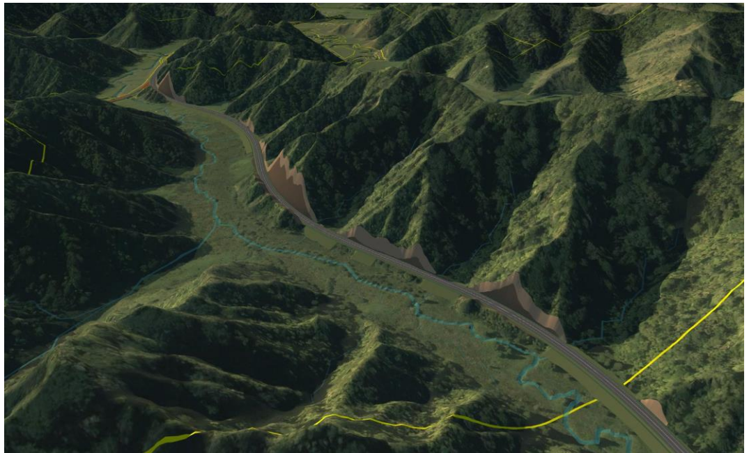
Figure 31: Shading of the road in the Mangapepeke Valley at 2:00pm, mid-winter
