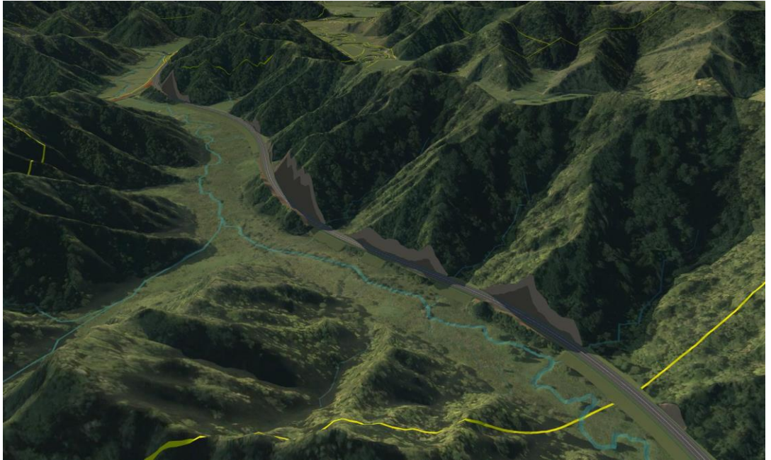
Figure 30: Shading of the road in the Mangapepeke Valley at noon, mid-winter
