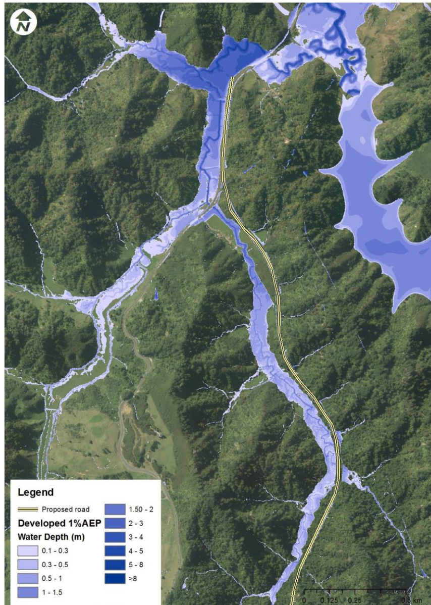
Figure 32: Flood depths during a 1% AEP design rainfall event for the proposed developed road scenario in the Northern catchment.
