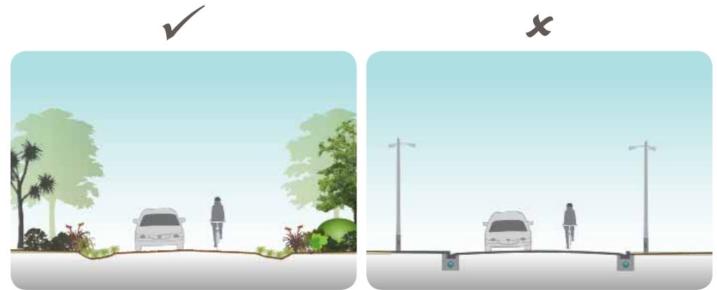
Above: Carriageway widths should be as narrow as possible to increase safety and efficiency and control vehicle movement and speeds. Permeable materials like gravel reduce the volume of stormwater.
