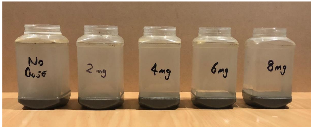
Plate Three - Sample Jars Showing Settlement after 30 minutes for Soil Sample
