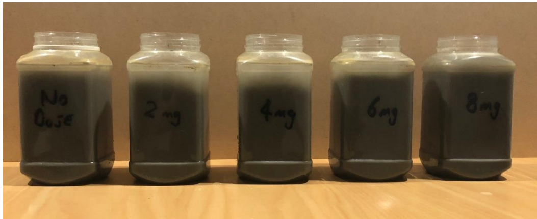
Plate Two - Sample Jars Showing Settlement after immediate mixing for Soil Sample
