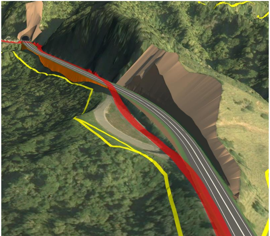
Figure 14: MCA2 - Online Z Option: Northern tunnel portal showing large extent of the Z option retaining wall structure (orange) along the existing alignment (red) which will create significant delays to existing traffic during construction.
