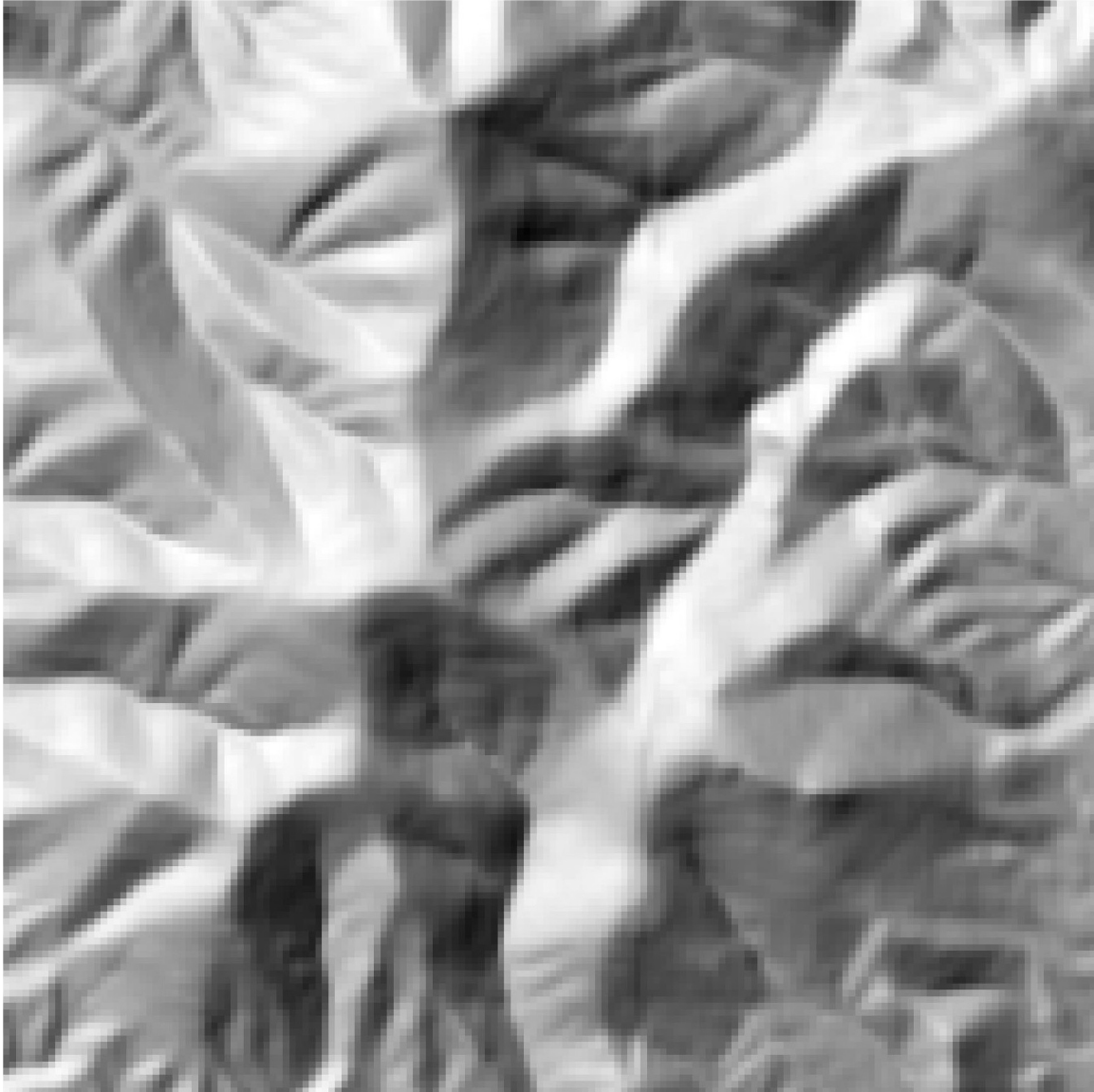
Figure 14. A hillshaded map of the Sweet Grass Hills of north-central Montana using 256 shades of gray.
