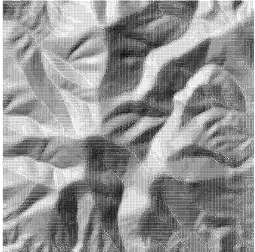
Figure 18. The same hillshaded map in Figure 15 dithered with the halftone patterns from Figure 10 oriented perpendicular to the aspect direction.
