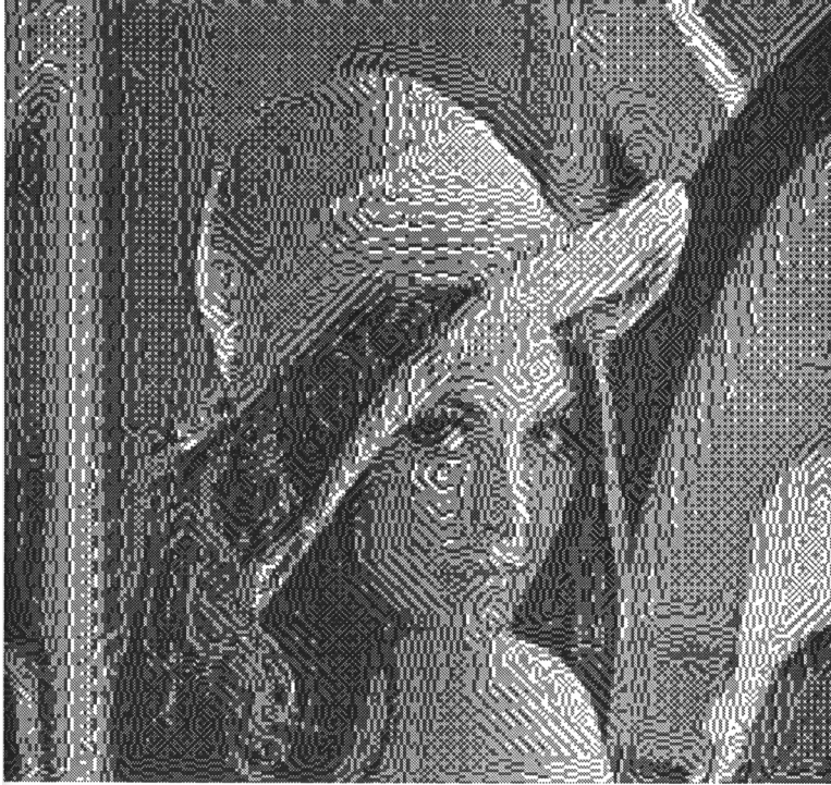
Figure 8. An image with halftones oriented in the direction of gradient of gray values (From Sloan and Wang (1992) with permission from SPIE).
