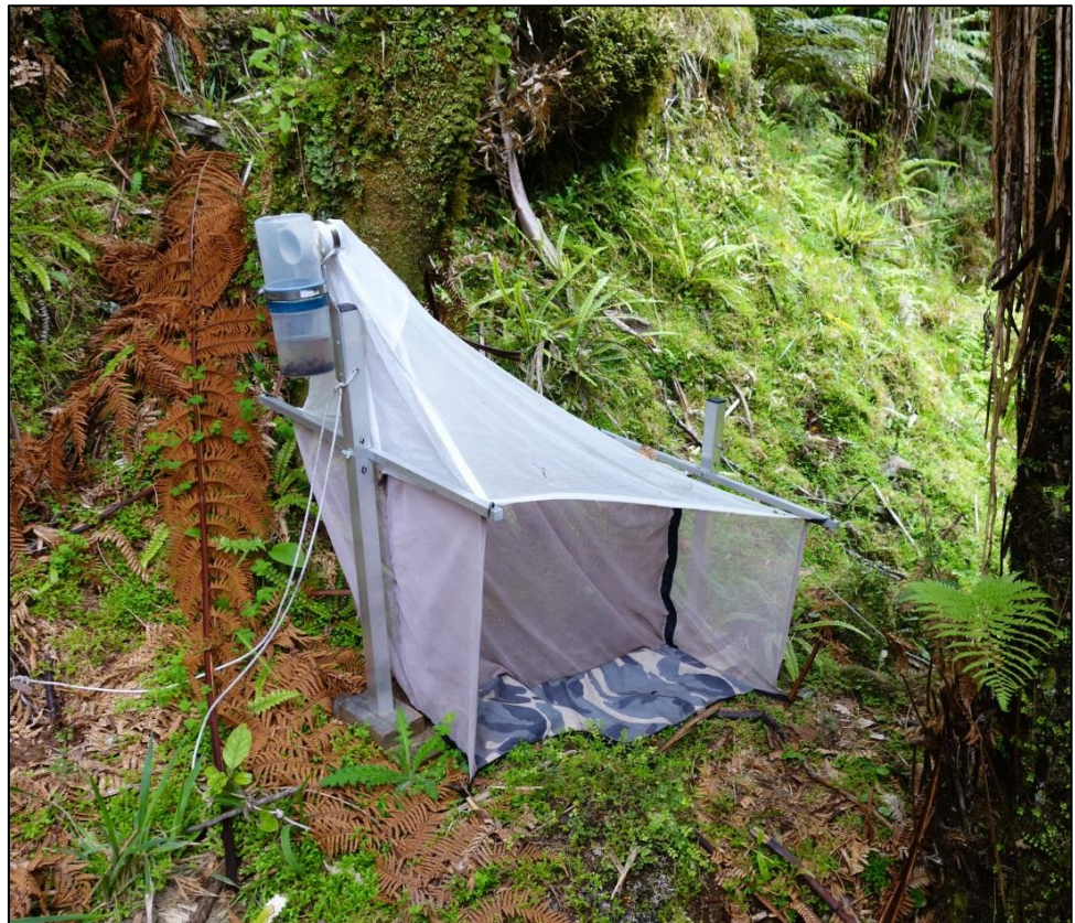
Figure 2. A malaise trap used to collect flying insects, particularly flies, wasps and beetles.
