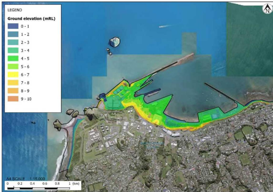
Figure 3.13: Ground surface elevations less than 10 m RL (NZVD 2016) around Port Taranaki.
