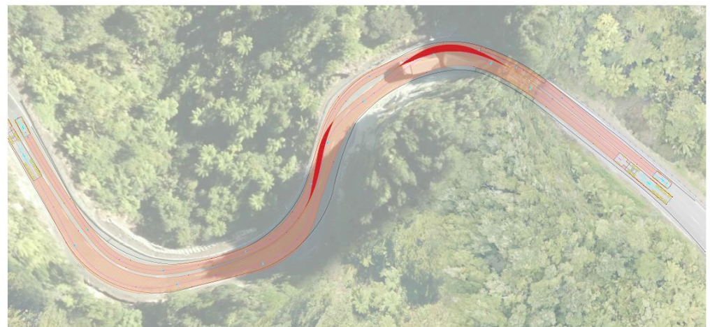
Figure 8 - Northbound semitrailer and southbound 99% car through Mt Messenger tunnel
