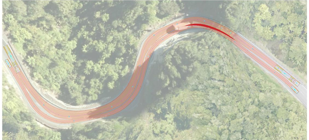
Figure 7 - Southbound semitrailer and northbound 99% car through Mt Messenger tunnel
