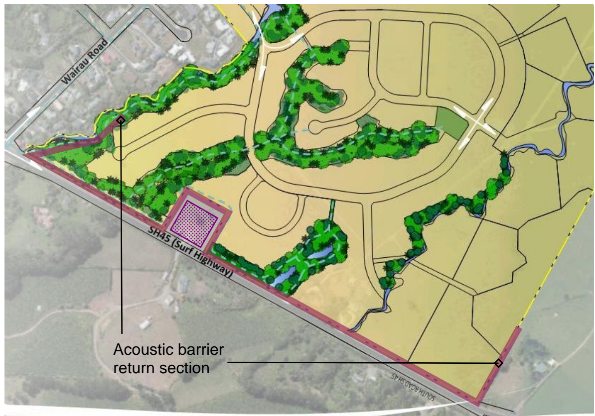
Figure 2: Noise barrier location
