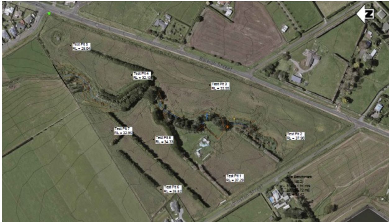
Figure 5 – Extract from draft hand auger location plan by Civil Infrastructure Consultants Ltd (drawing attached in Attachment A). Note that the reference to “test pits” is erroneous – we understand that all investigation locations were hand augers.
