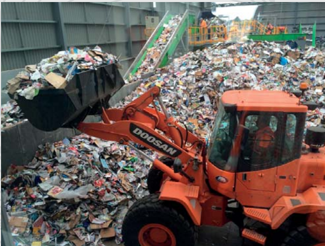
PHOTO 4: Recyclables being placed on the sorting line at the MRF
