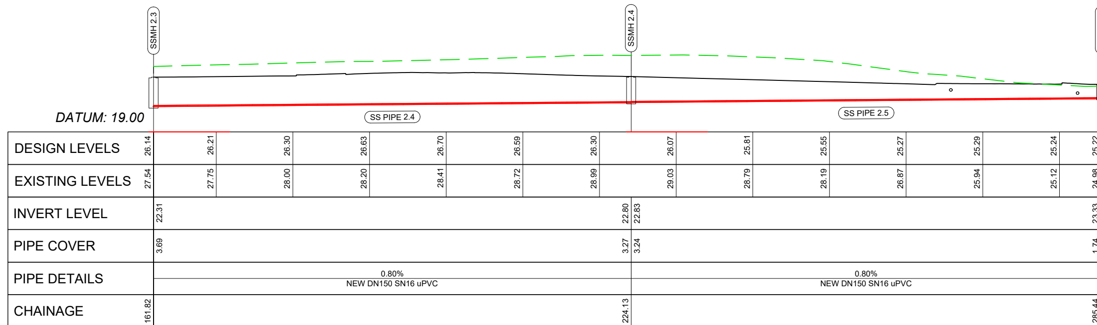
SEWER PROFILE - SSMH 2.3 - SSMH 2.5 SCALE - HORIZONTAL 1:500 VERTICAL 1:500
